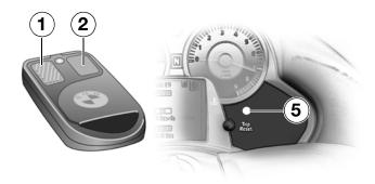
Once the immobiliser has been activated the engine will refuse to start even if an authorised key is used for the start attempt. You can tell whether the immobiliser is activated by switching on the ignition and observing LED 5; if the immobiliser is active it will light up when the pre-ride check completes.
