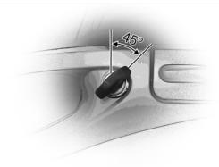
If the compartments were locked by the central locking system and, for some reason, the remote control unit is not to hand, you can use the emergency unlocking routine to open them. Emergency unlocking is independent of the current status of the lock barrel. You cannot use the emergency unlocking routine to open the radio compartment.
